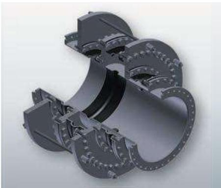
Pressure Balanced Rubber Expansion Joint 3D modelling.
