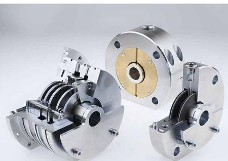
Carbon floating ring seals are supplied as maintenance-free compact labyrinth cartridge seals with low leakage. The floating self-adjusting sealing rings provide radial sealing on the shaft with a very small gap. The seal requires no additional lubrication, and it is designed for dry running. Besides pure gas, carbon floating ring seals are also suitable for Atex applications, toxic media, media containing solids, flue gas, dust, powder, vapor, liquid mist, oil mist and penetrating oil.
