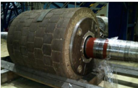
UPM Plattling/Germany uses Metso pressure grinders to fiberize wood. EagleBurgmann **HSSHR8-D4/470-E1** type mechanical seals are used to seal off both sides of the high-consistency groundwood pulp at the grindstone shaft. Operating conditions:  $p = 3 \text{ bar (44 PSI)}$ ,  $t = 150 \text{ }^\circ\text{C (302 }^\circ\text{F)}$ ,  $n = 350 \text{ min}^{-1}$ .
