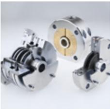
Carbon floating ring seals are supplied as maintenance free compact labyrinth cartridge seals with low leakage. The floating self-adjusting sealing rings provide radial sealing on the shaft with a very small gap. The seal requires no additional lubrication, and it is designed for dry running. Besides pure gas, carbon floating ring seals are also suitable for Atex applications, toxic media, media containing solids, flue gas, dust, powder, vapor, liquid mist, oil mist and penetrating oil.
