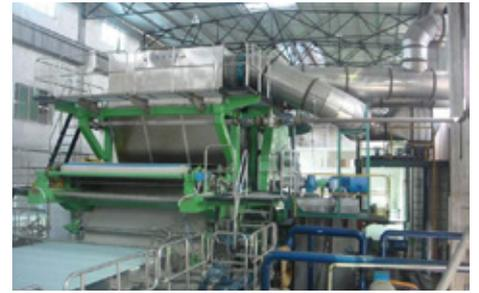
A **Yankee Flex 350** type fabric expansion joint with an outer layer of Alusil is installed in an air duct system at the paper mill of Procter & Gamble Paper in Oxnard, USA. The expansion joint is reliably tight and flexible. Operating conditions:  $t = 343 \text{ °C}$  (649 °F), rate of flow = 15 m/s (49 ft/s).
