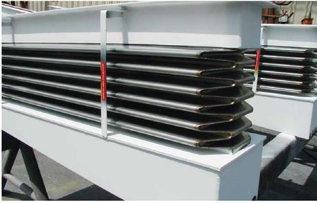
**Expansion joints** with specially shaped edges are installed in an air preheater at East Kentucky Power in the US. Operating conditions:  $p = 0.07 \dots 0.24 \text{ bar}$  (1.02 ... 3.48 PSI);  $t = 34 \dots 540 \text{ °C}$  (640 °F ... 1,004 °F).
