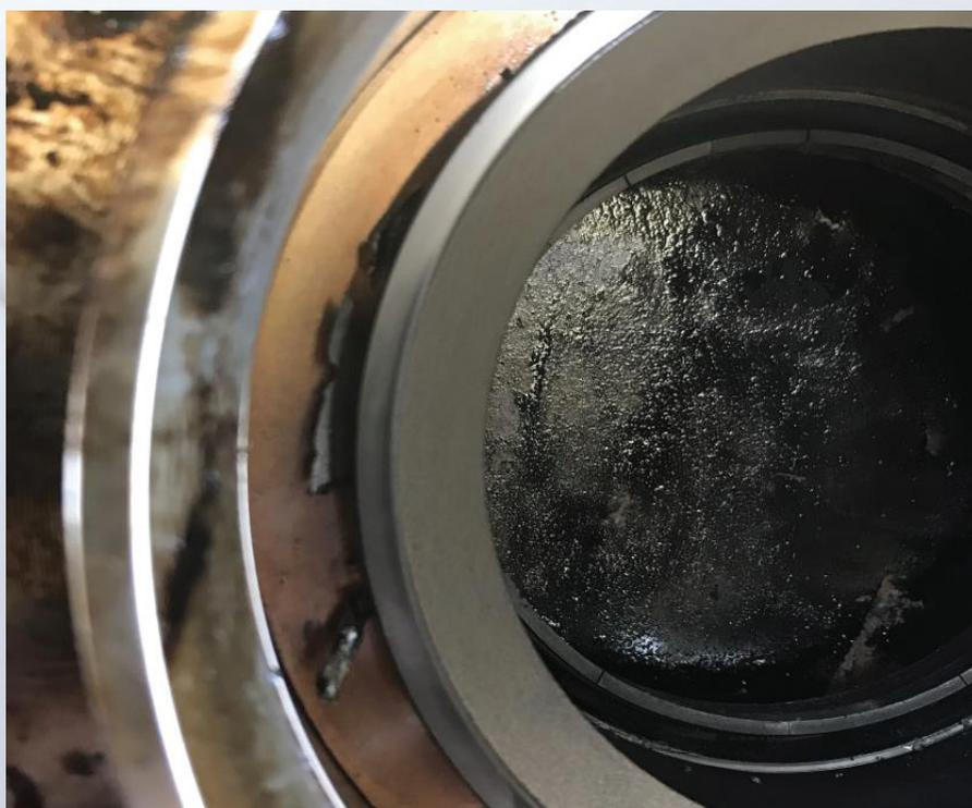
Despite phases without flushing, the DiamondFace sliding faces were still in top condition after 18 months.
