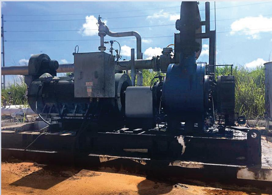
Multiphase pumps are used for extra-heavy crude oil production.
