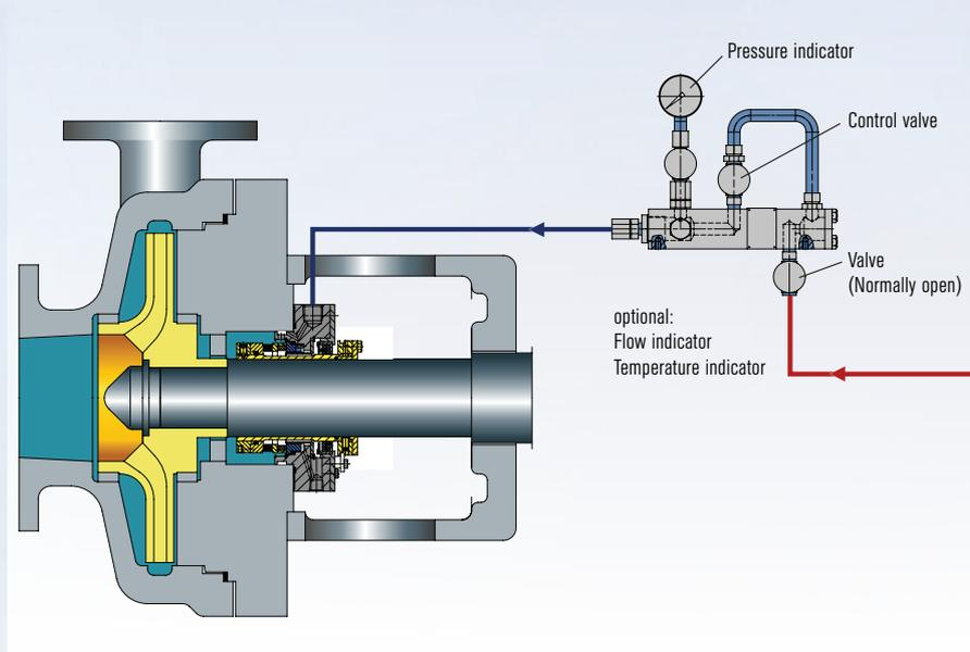
API plan 32: Flush fluid is injected into the seal chamber from an external source.
